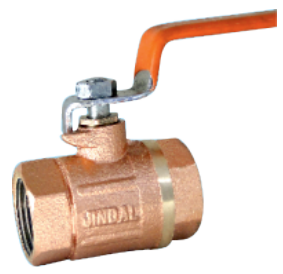
G.M. Ball Valves (Medium) with M.S. Ball & Teflon Seat Tested 300 lbs. Size : 15mm to 50mm
